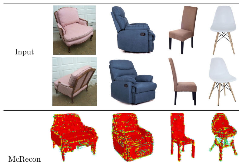
Figure 3.7: Qualitative results of multi-view real image reconstructions on Stanford Online Product dataset [38]. Our network successfully reconstructed real images coordinating different views.
