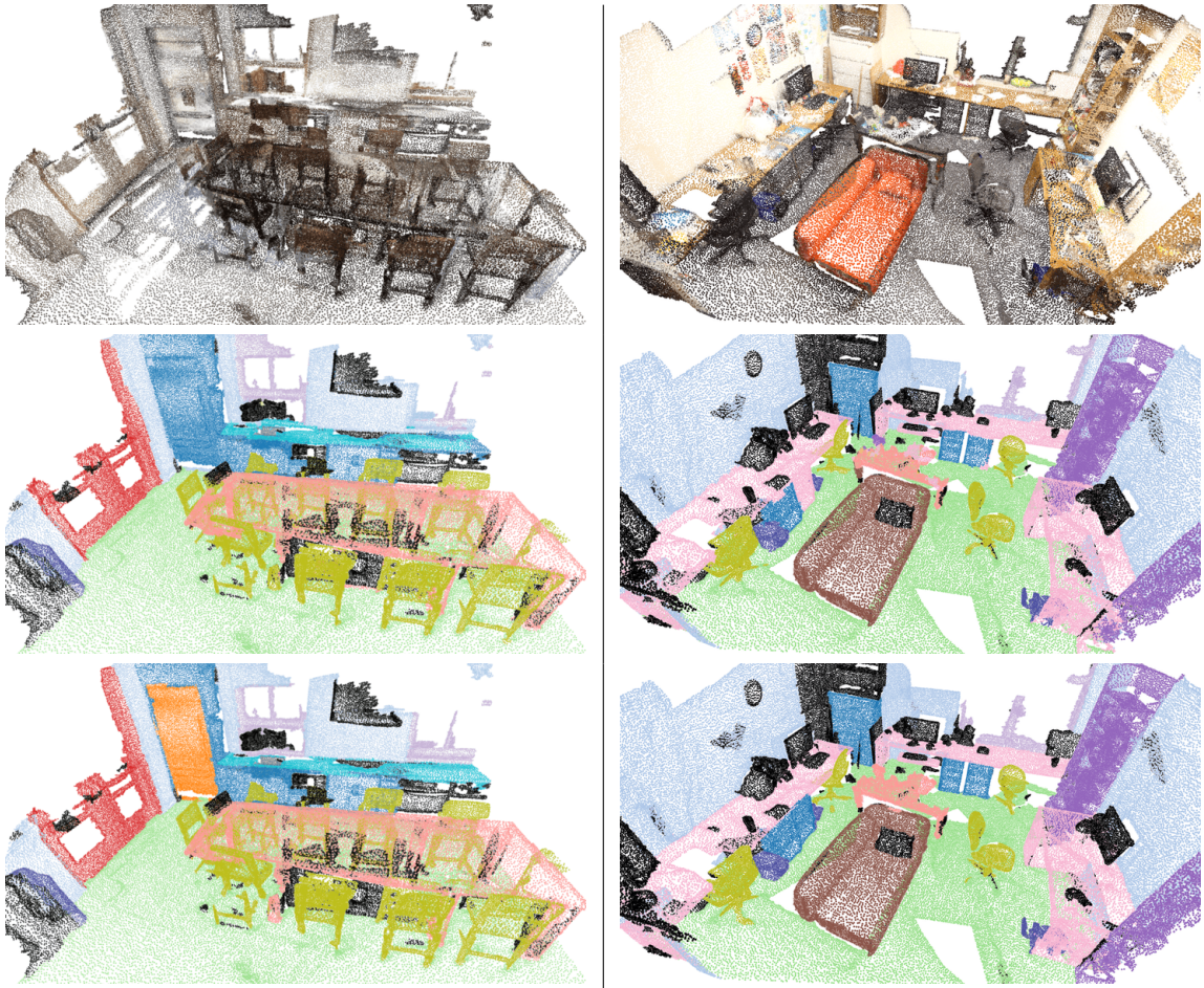
Figure 5.8: Visualization of Scannet predictions. From the top, a 3D input pointcloud, a network prediction, and the ground-truth.
